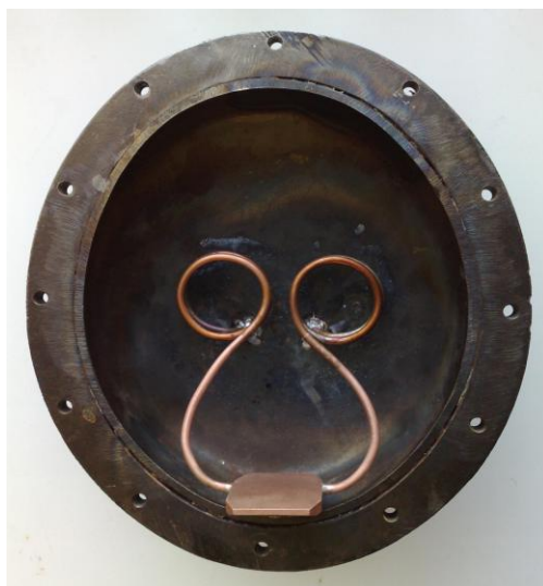
Figure 6. PLT evaporator and transport zone with two pipes for vapor and liquid transport between the evaporator and condenser
